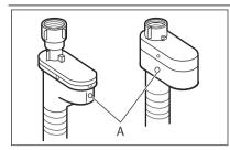
The inlet hose has a water stop device. This device prevents water leaks in the hose because of its natural ageing. The red sector in the window «A» shows this fault.
